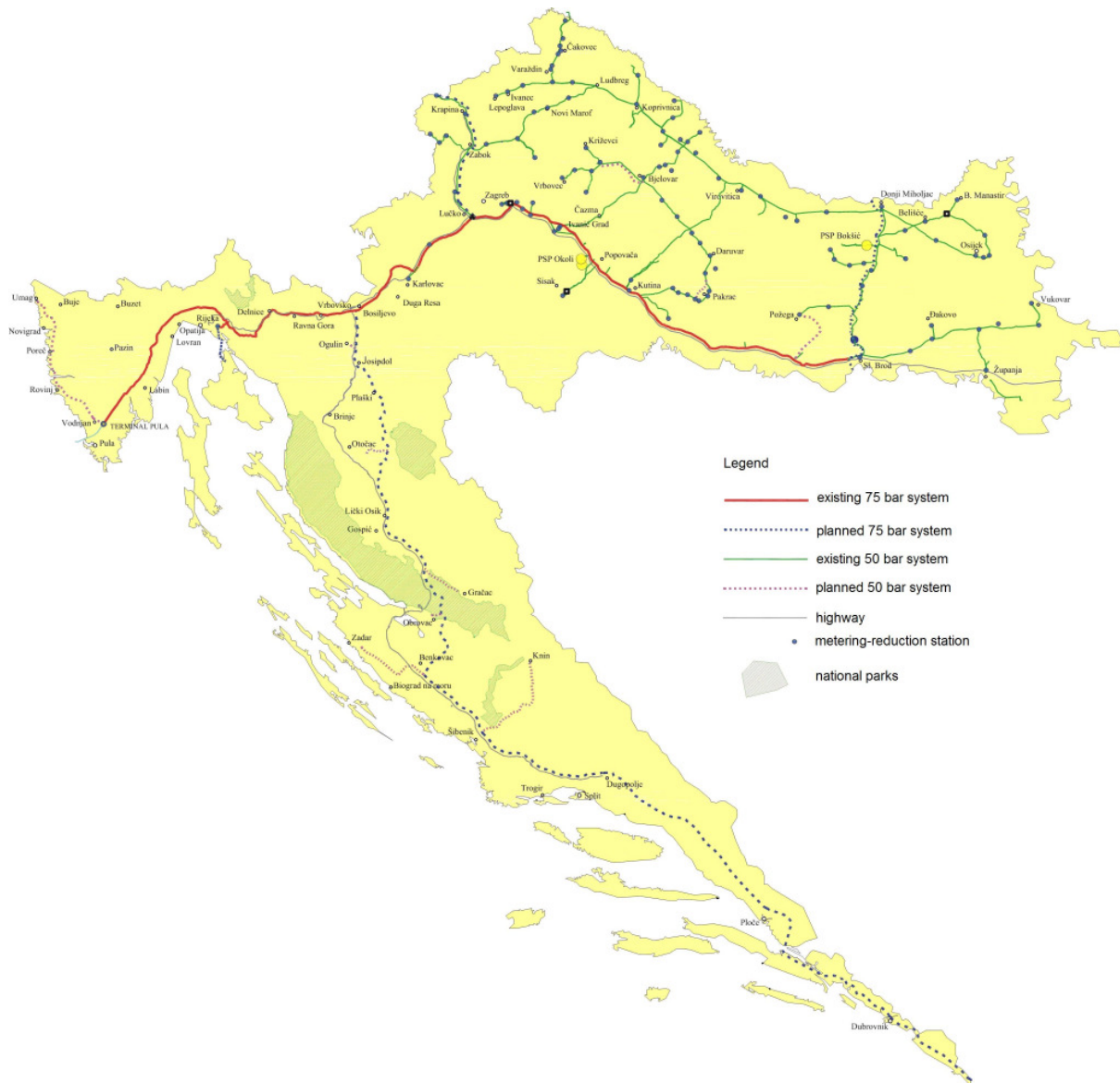
Illustration 14: Croatian gas transportation system; Source: EIHP
